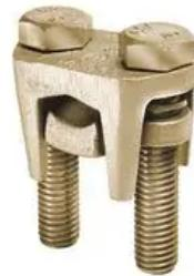
Compact, two-piece, high strength, high copper alloy BURNDY OKLIP recommended for heavy duty connections. Neoprene rings hold DURIUM bolts in place during installation. Installed with ordinary wrench. Recommended tightening torque: 325 in-lb.
